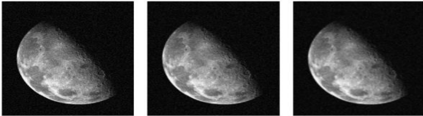
Figure: Input image; Mean image with 3 × 3 kernel and Mean filter with 5 × 5 kernel.
